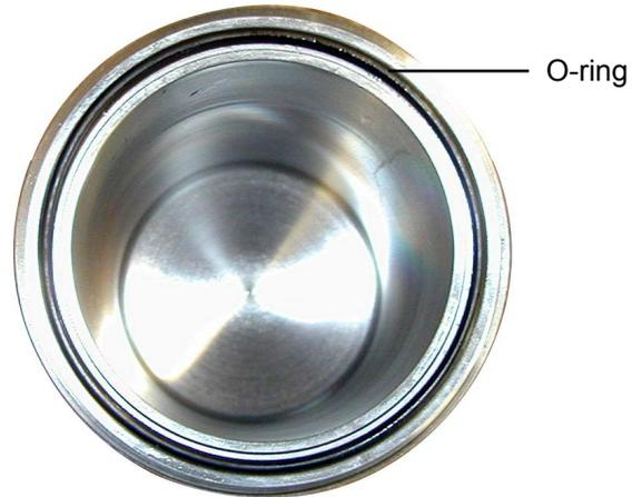
2. Determine a safe volume and safe initial pressure for the temperature at which the sample will be tested (refer to the chart on page 5). Place the correct volume of fluid into the cell. Be careful not to get fluid in the o-ring groove or on the o-ring.
