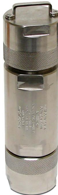
8. Place the assembled cell into a Curing Chamber, autoclave, or bath.
